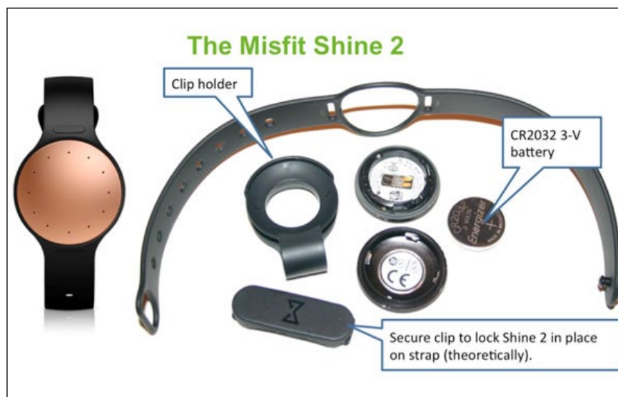
Figure 1. It's sleek design and ability to go 6 months on a single CR2032 3V coin cell battery made the Misfit Shine 2 an EDN teardown target at DesignCon.
