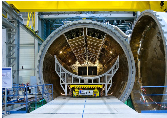
Figure 1. The omniMove mobile platforms from KUKA for extremely heavy loads of up to 100 tonnes, are used e.g. in aircraft construction.
